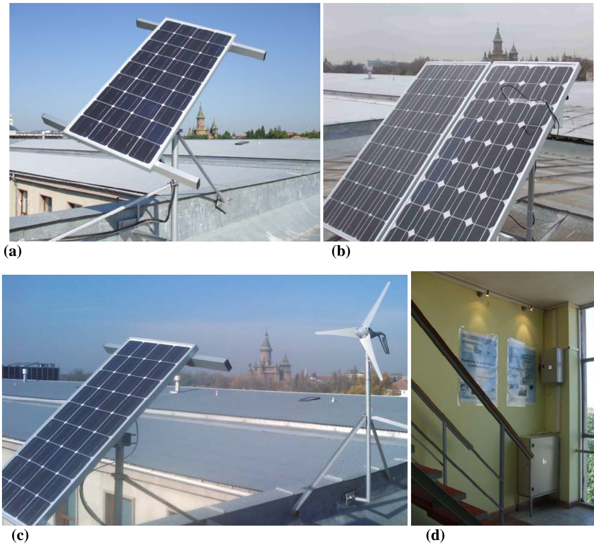
Figure 4. (a) PV-mobile system; the PV module is mounted on a polar axis sun tracker support; (b) PV-fix and PV-test modules. On front of PV-test module it can be seen the pyrometer measuring the cells temperature; (c) Wind generator (d) View of the PV-LAB components inside: (a) Electric block including the instruments for monitoring PV-mobile and PV-fix systems; (b) Battery block. The loads consisting of two 20W spots (upper side of the photo) are used directly for illumination.
