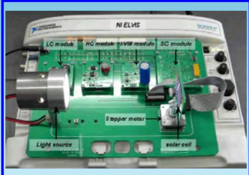
$$I = I_{ph} - I_o \left( e^{\frac{V+IR_s}{nV_T}} - 1 \right) - \frac{V + IR_s}{R_{sh}}$$
